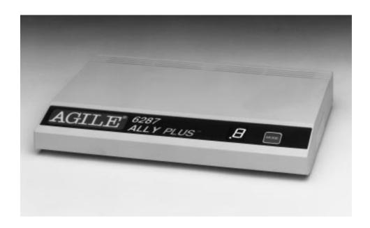
The AGILE 6287 ALLY PLUS is a high-performance, feature-rich, printer interface that enables an IBM mainframe computer system to print to industry-standard ASCII and EBCDIC printers. The ALLY PLUS has an RG62 A/U coax input port for connection to an IBM mainframe with a 3174, 3274 or 3276 establishment controller or a display/printer adapter.
